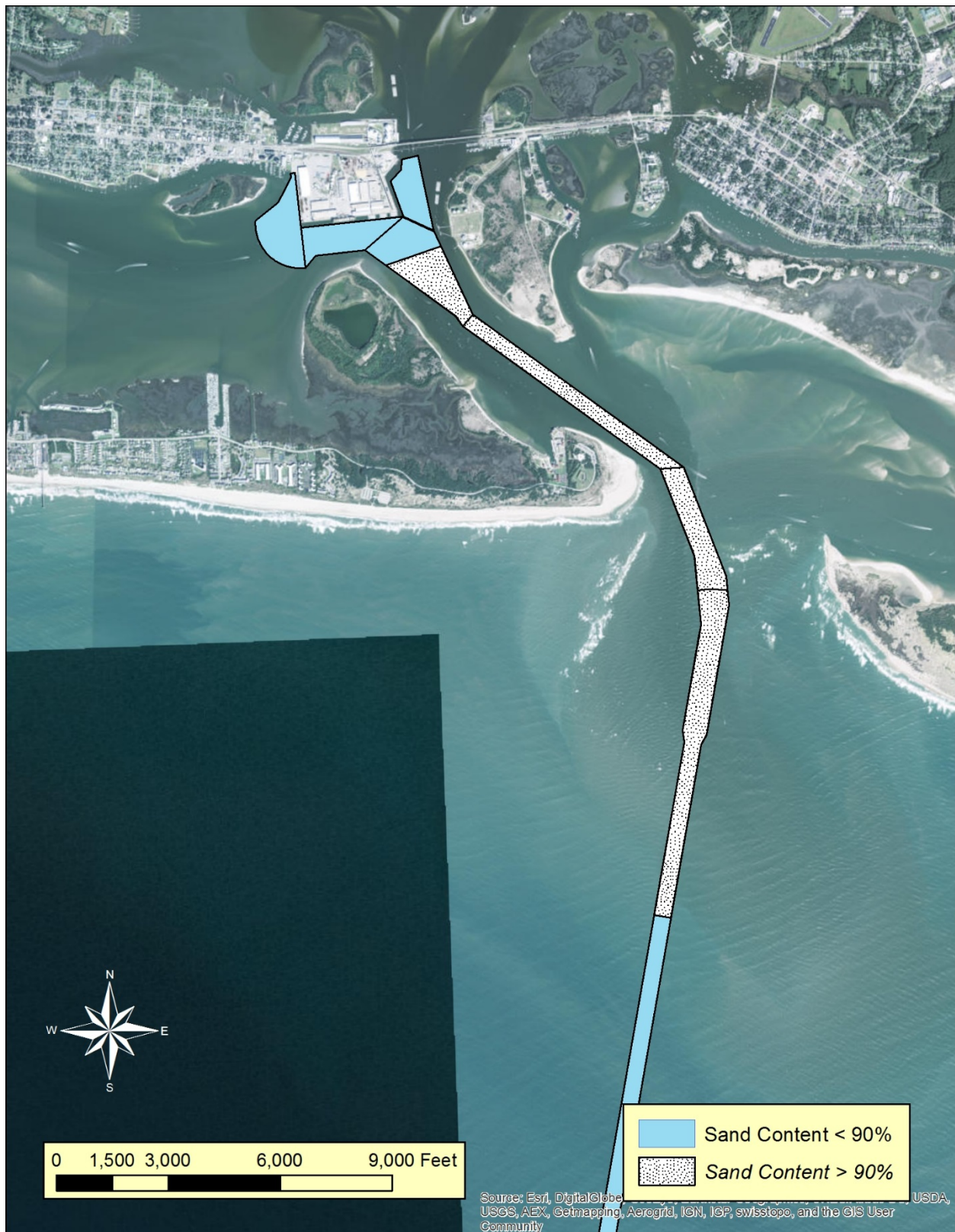
Figure 3-27. Inner/Outer Harbor Dredged Material Separation Based on Percent Sand
