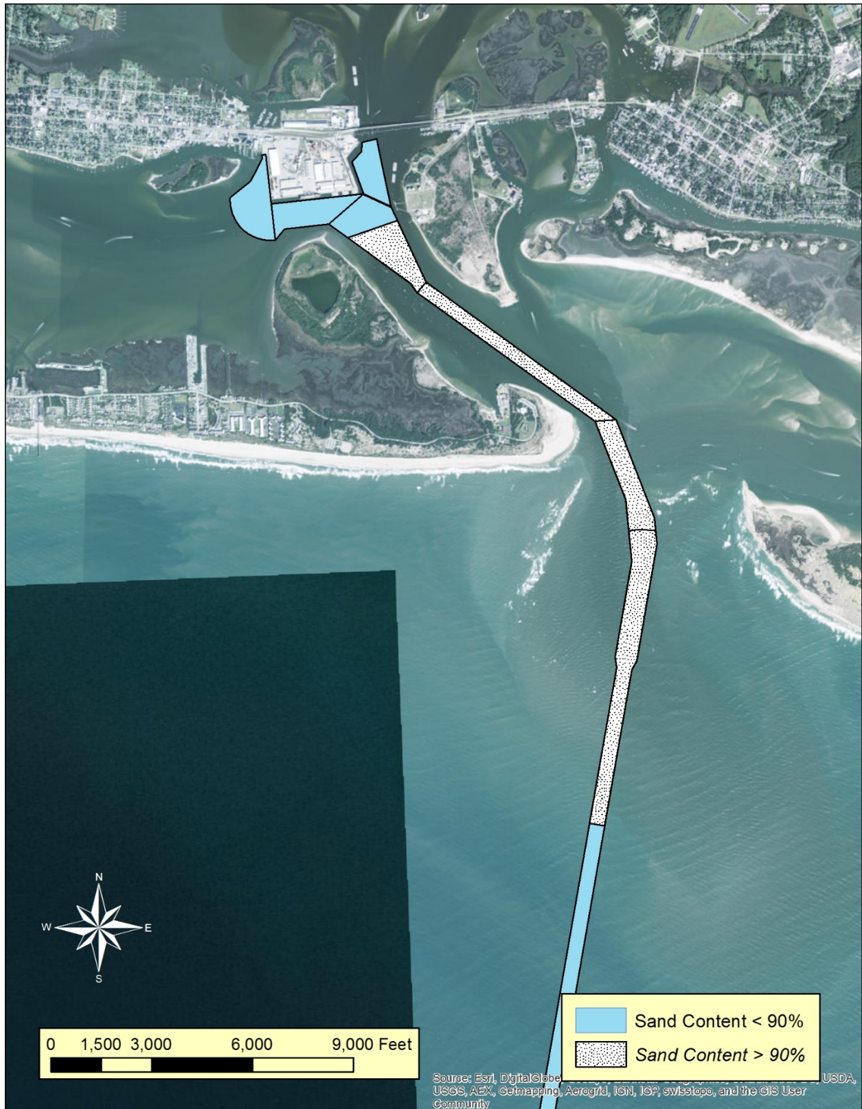
Figure 6. Morehead City Harbor Dredged Material Separation Based on Percent Sand
