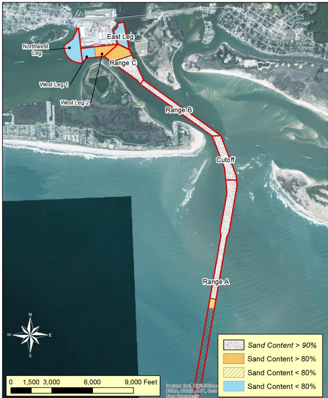
Figure 2-2. Inner/Outer Harbor Dredged Material Separation Based on Percent Sand
