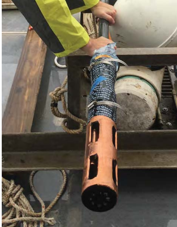
Photograph 1: Antifouling measures applied to EXO sonde
