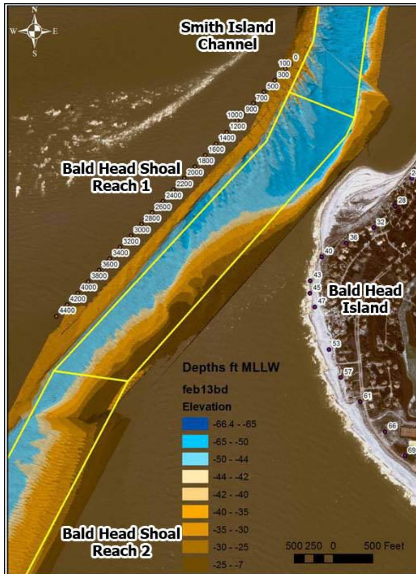
Figure 3.2. Entrance channel alignment near Bald Head Island, showing 3 years of shoaling that occurred prior to it being dredged in 2013.
