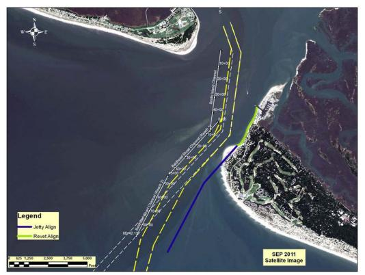
Figure 5.1. Conceptual alignment for a Bald Head Island jetty feature.
