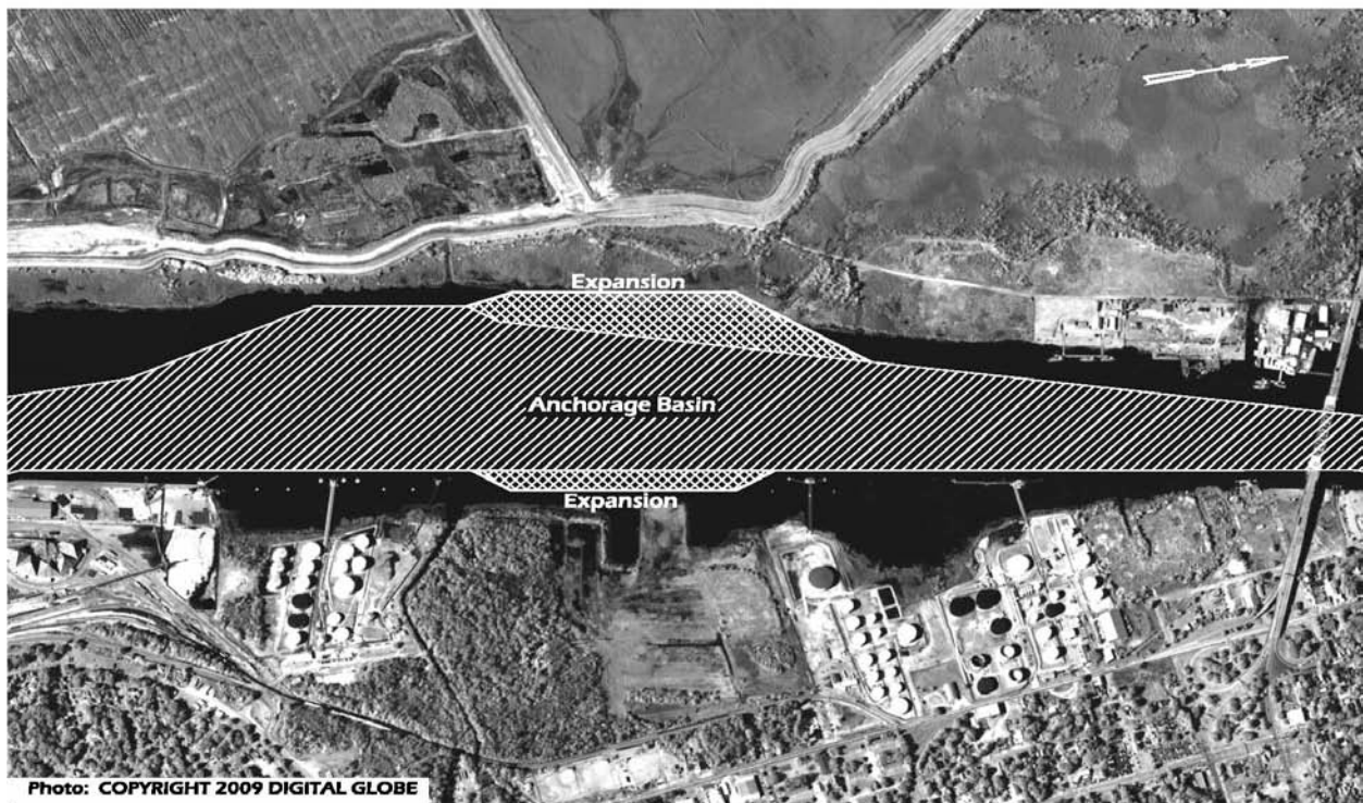
Figure 3. Anchorage (Turning) Basin Expansion
