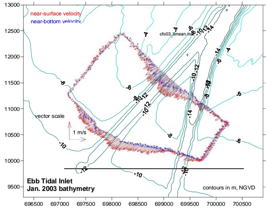
Figure 4.35 March 2003 ADCP survey at offshore transect during ebb flow.
