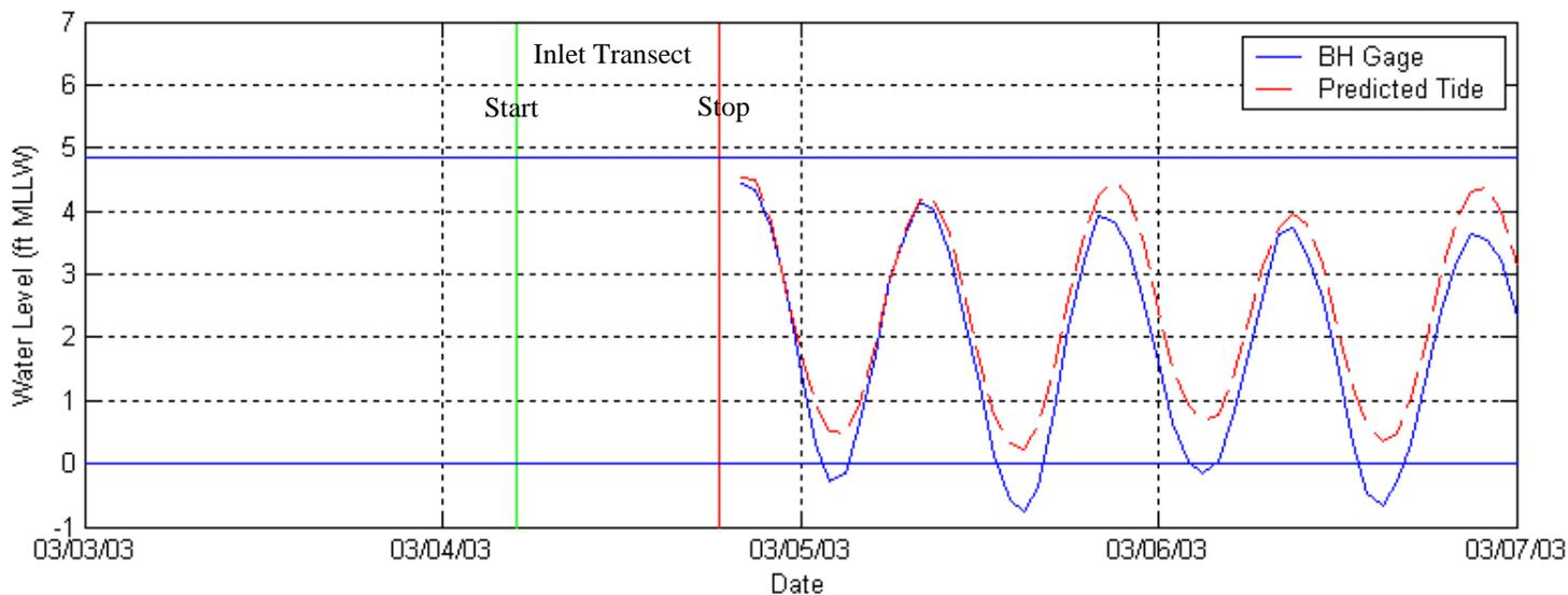
Figure 4.19 Predicted and observed water levels during the March 2003 ADCP survey (Inlet Transect)
