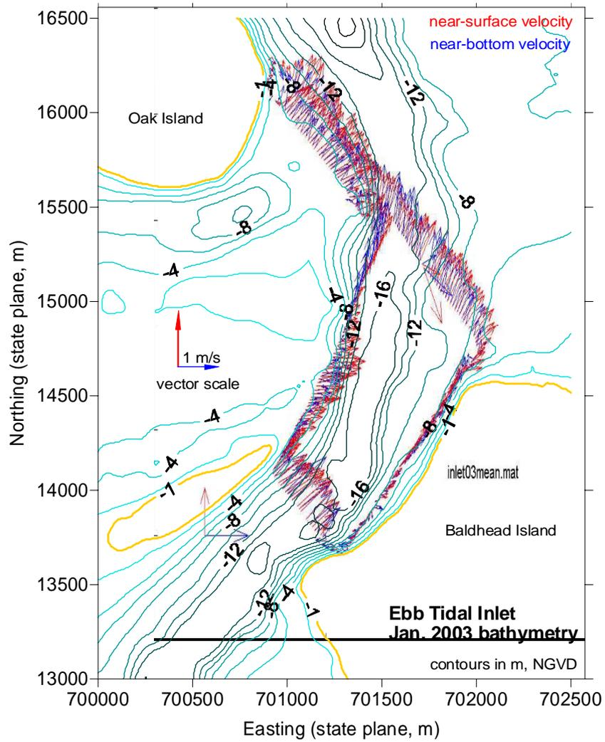
Figure 3.56 Peak flood current velocities at inlet transect for March 2003 ADCP survey
