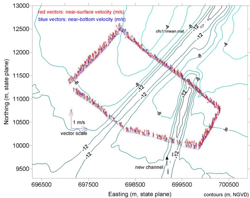
Figure 4.36 April 2002 ADCP survey at offshore transect during flood flow.
