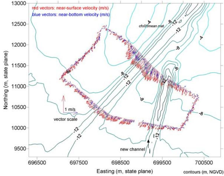
Figure 3.53 Peak ebb current velocities at offshore transect for April 2002 ADCP survey
