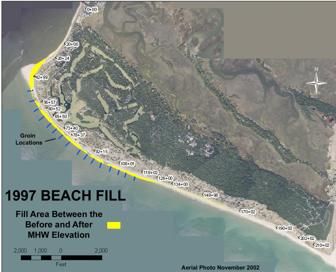
Figure 4.8 1997 Beach Fill with Geotextile Groins.
