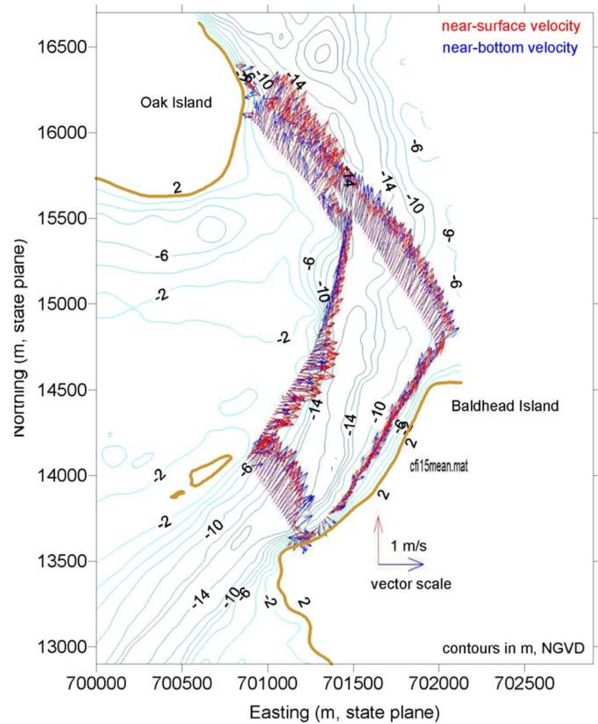
Figure 4.22 April 2002 ADCP survey at inlet transect during peak flood flow. Note that survey transect does not cover same area as the October 2000 survey.
