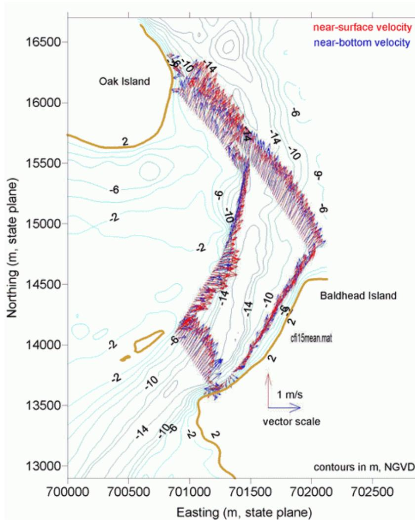
Figure 4.32 April 2002 ADCP survey at inlet transect during flood flow.
