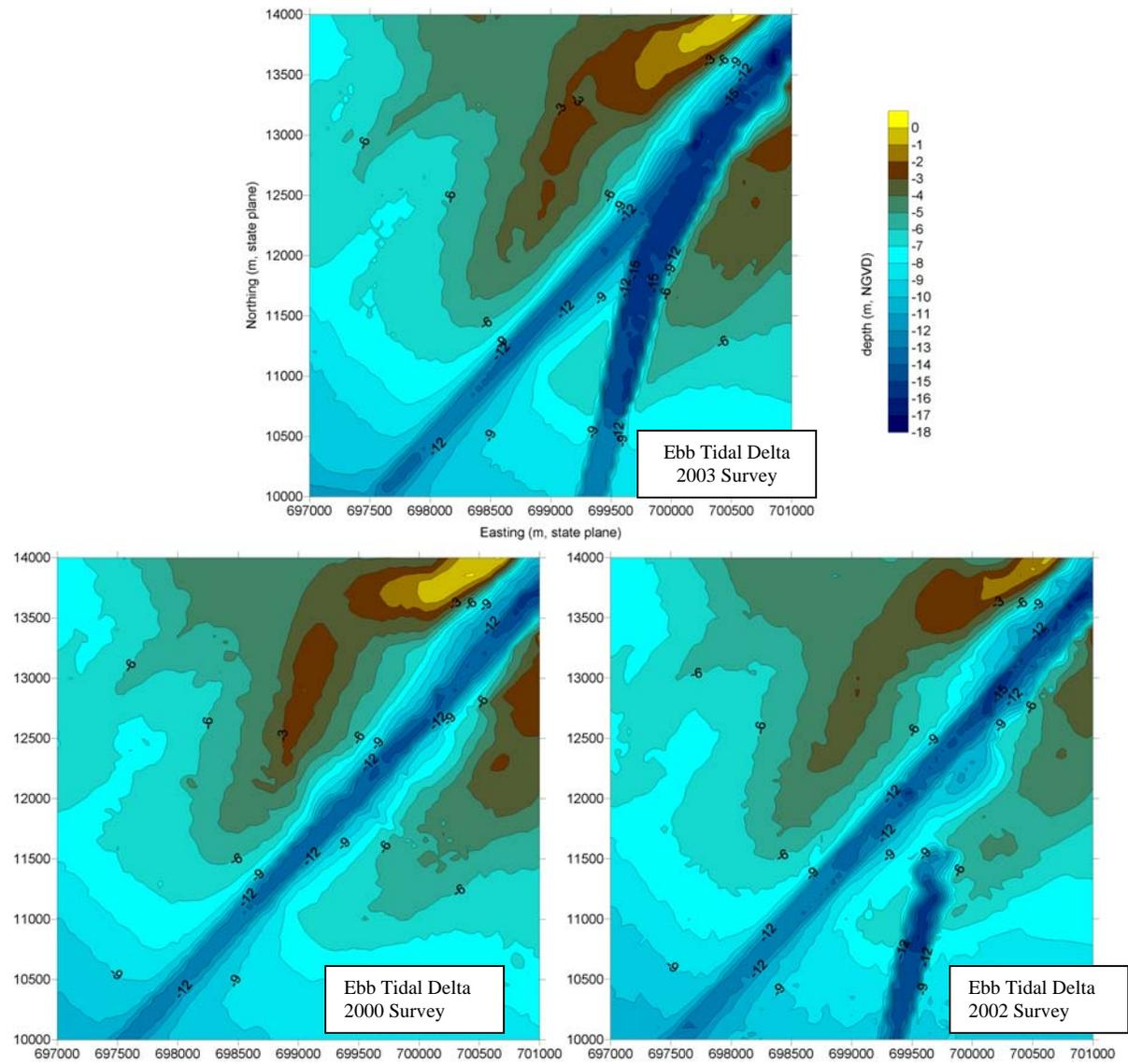
**Figure 3.22 Inset of bathymetry near the new channel from each of the three surveys- 2000, 2002, and 2003.**
