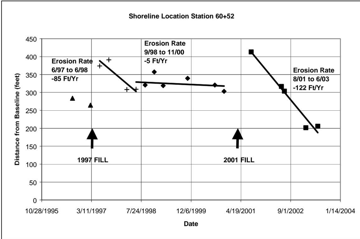
**Figure 4.9 Shoreline Locations and Erosion Rates for Station 60+52.**
