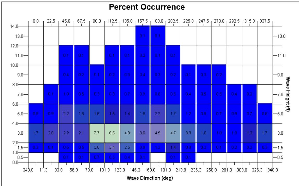
Figure 3.29. Wave Height Block Diagram for WIS Level 3 Station 317.
