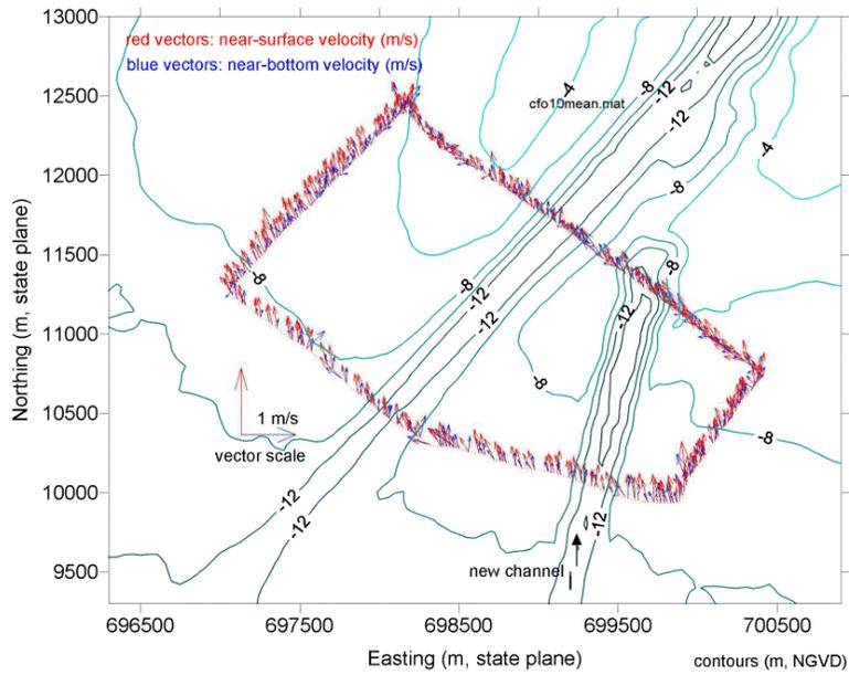
Figure 3.54 Peak flood current velocities at offshore transect for April 2002 ADCP survey
