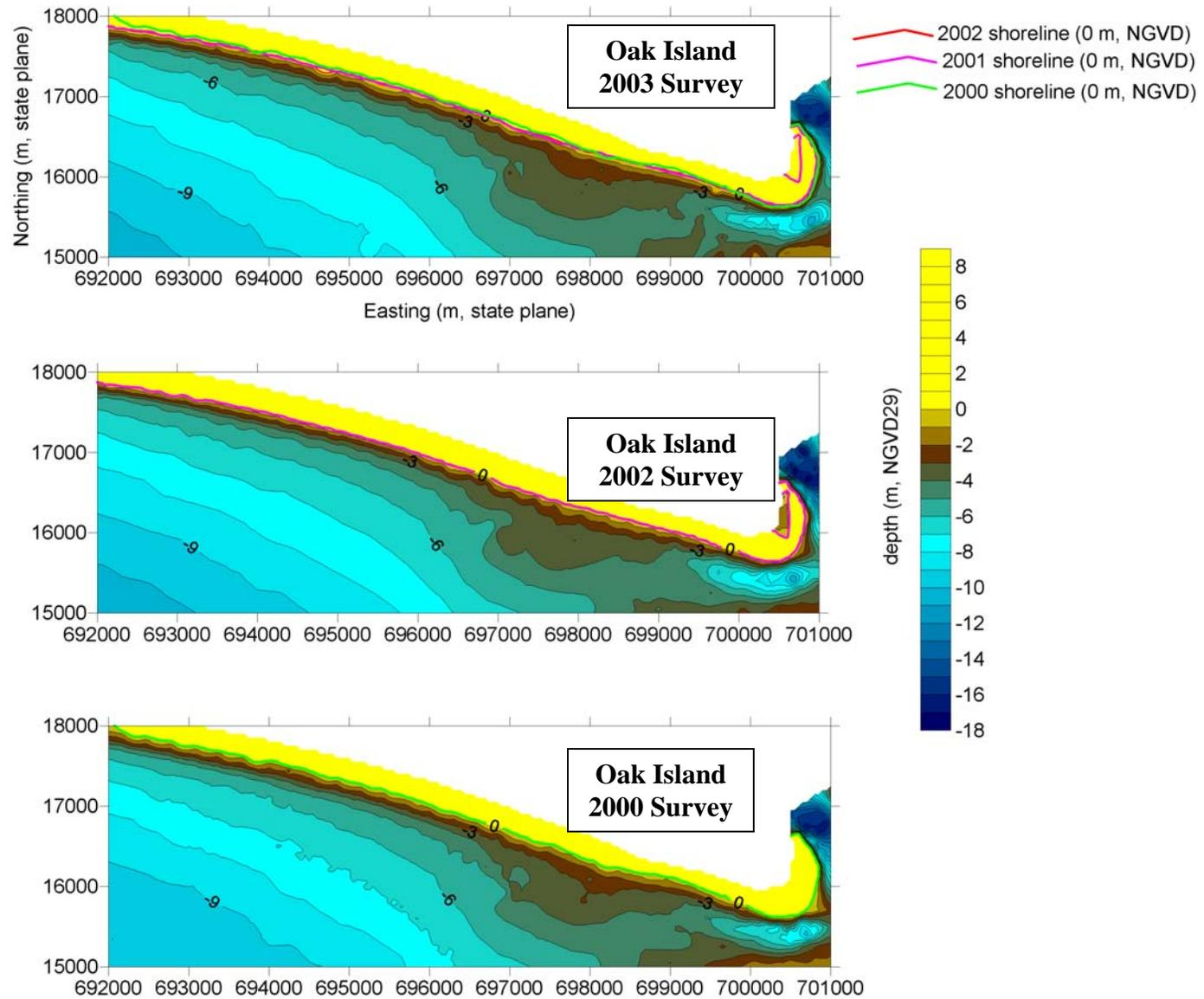
Figure 3.25 Comparison of bathymetry along the eastern portion of Oak Island from the 2000, 2002, and 2003 surveys.
