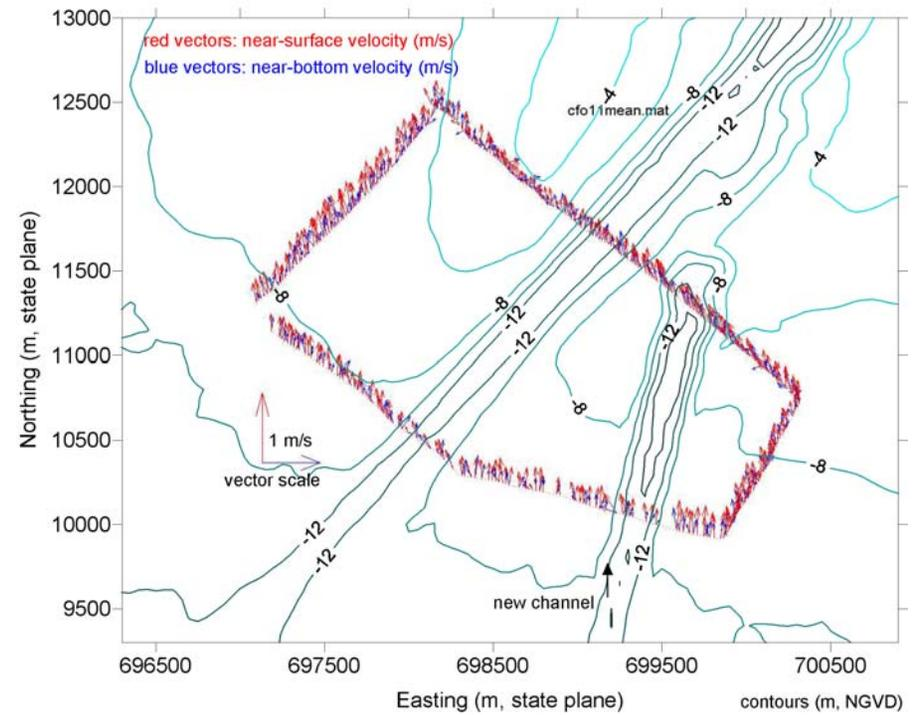
Figure 4.26 April 2002 ADCP survey at offshore transect during peak flood flow.
