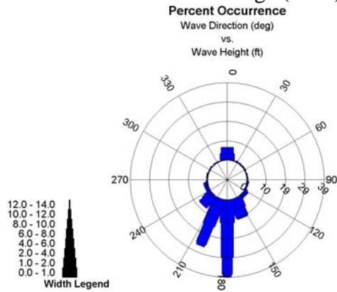
Figure 3.37 Wave Height Roses for FRF Gauges (2002).
