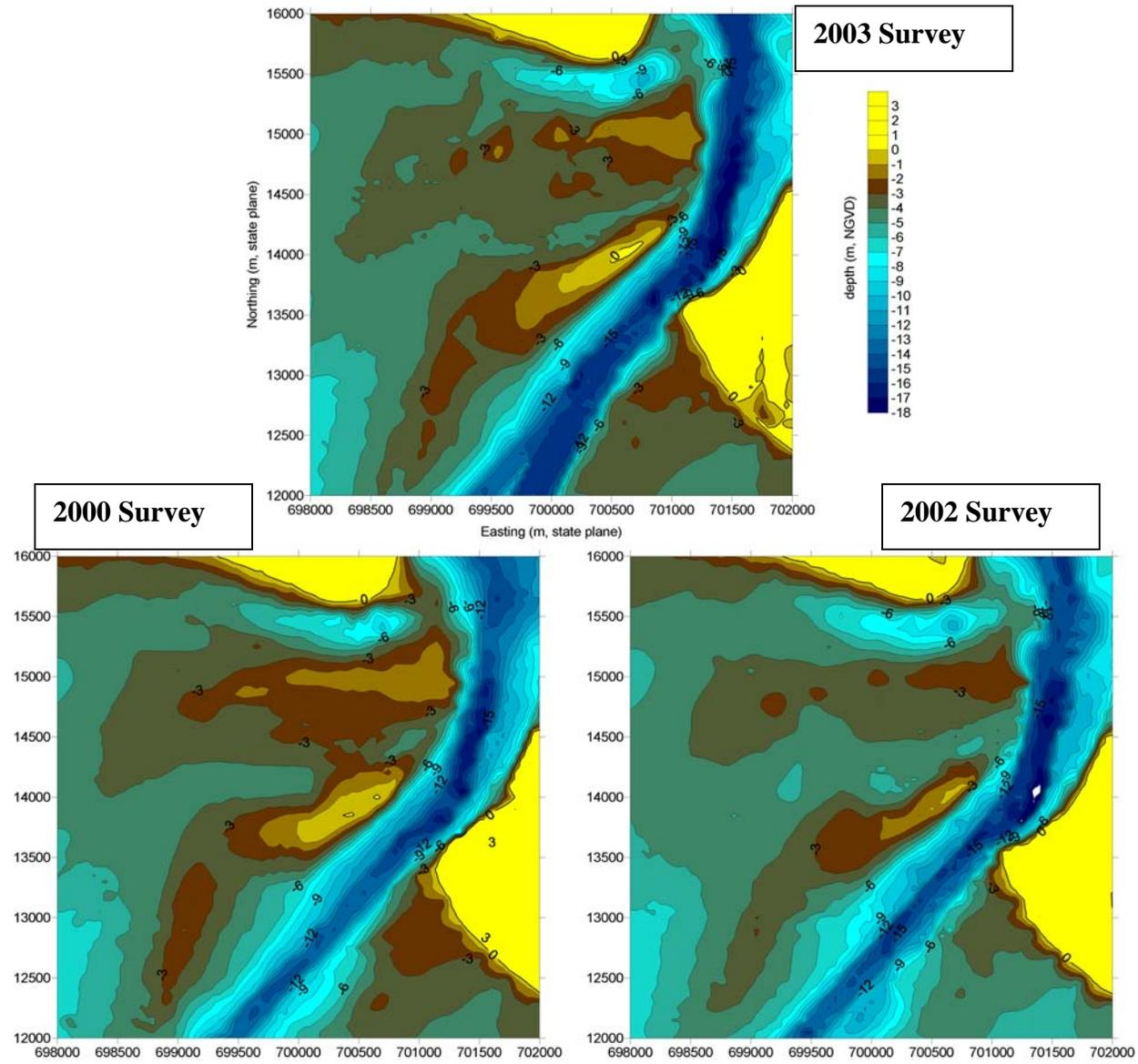
**Figure 3.20 Comparison of bathymetry near the Cape Fear River tidal inlet showing bathymetry from the 2000, 2002, and 2003 surveys.**
