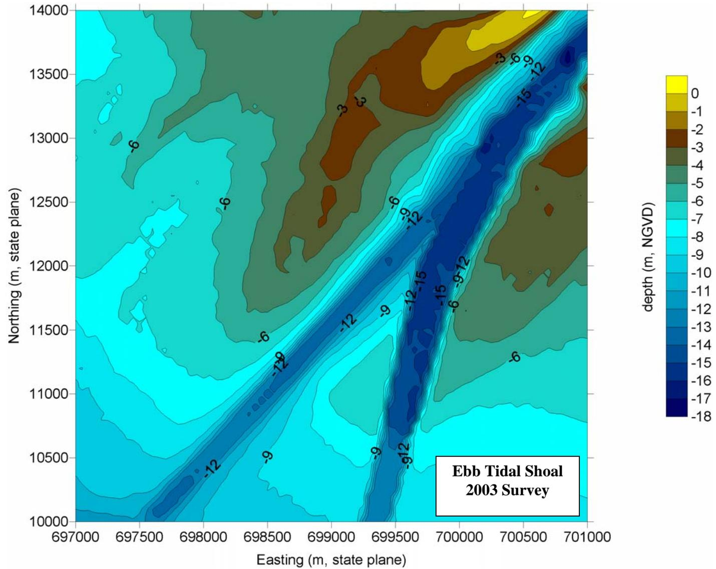
**Figure 3.21 Inset of bathymetry near the new channel along the distal end of the ebb tidal delta 2003.**
