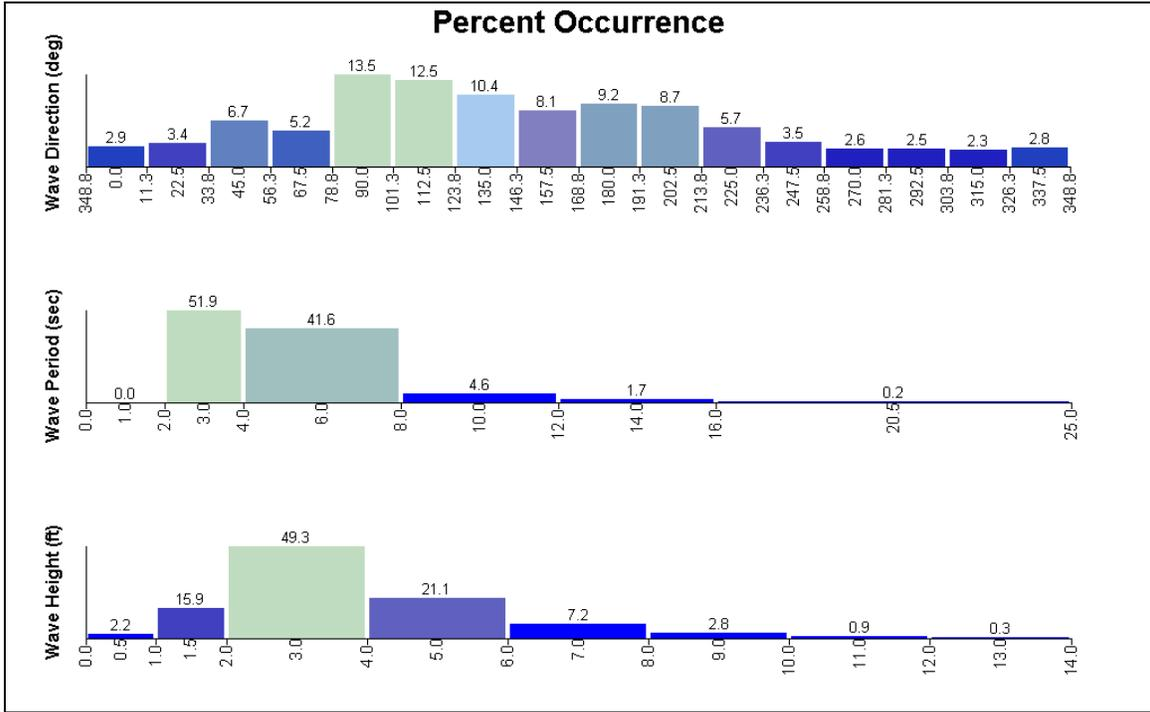
Figure 3.28. Wave Histogram for WIS Level 3 Station 317.
