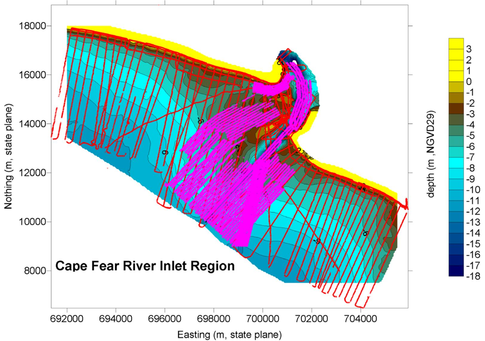
**Figure 3.17** Survey Track Lines Collected by the LARC5 and the Interferometric System during the 2003 Survey
