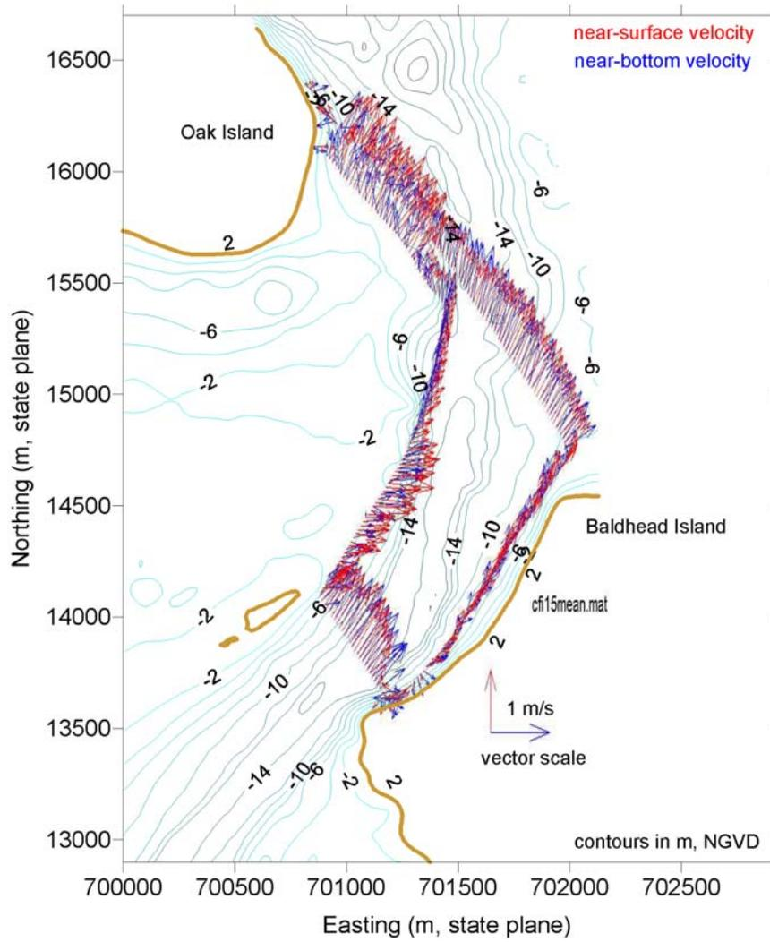
**Figure 3.52 Peak flood current velocities at inlet transect for April 2002 ADCP survey**
