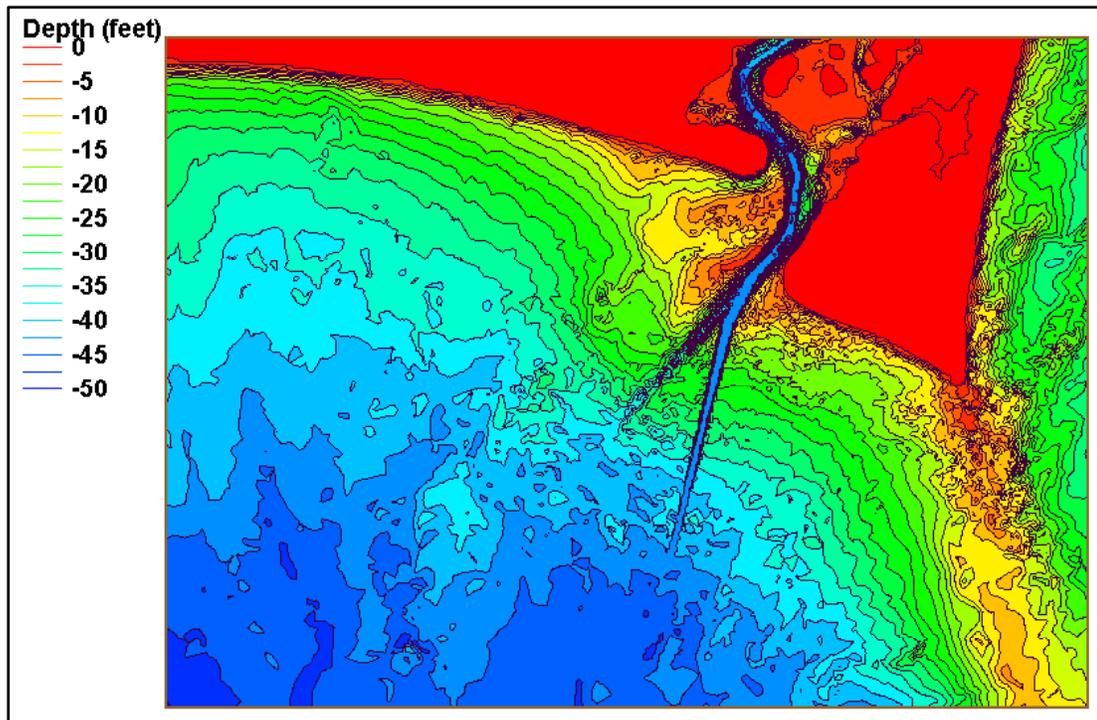
**Figure 3. 41 Cape Fear Bathymetry with Entrance Channel Plan.**
