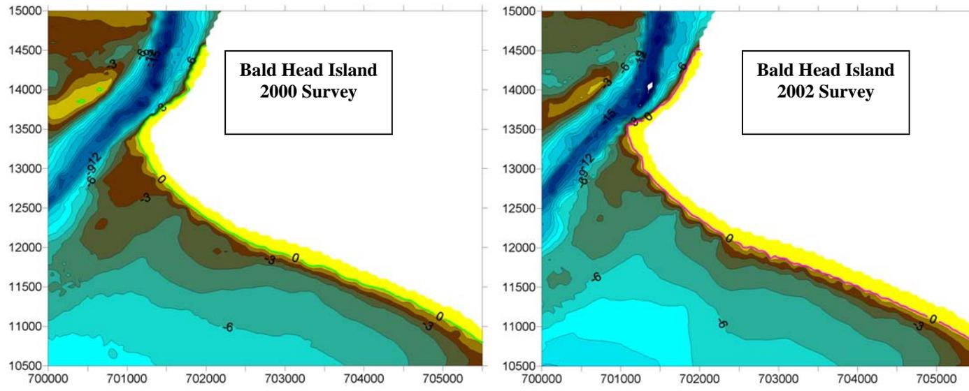
**Figure 3.24 Comparison of bathymetry along the western portion of Bald Head Island from the 2000, 2002, and 2003 surveys.**
