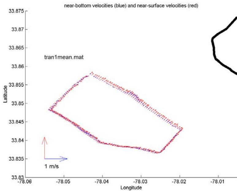
Figure 4.25 October 2000 ADCP survey at offshore transect during peak flood flow.
