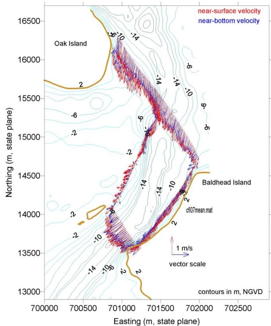
Figure 4.24 April 2002 ADCP survey at inlet transect during peak ebb flow. Note that survey transect does not cover same area as the October 2000 survey.
