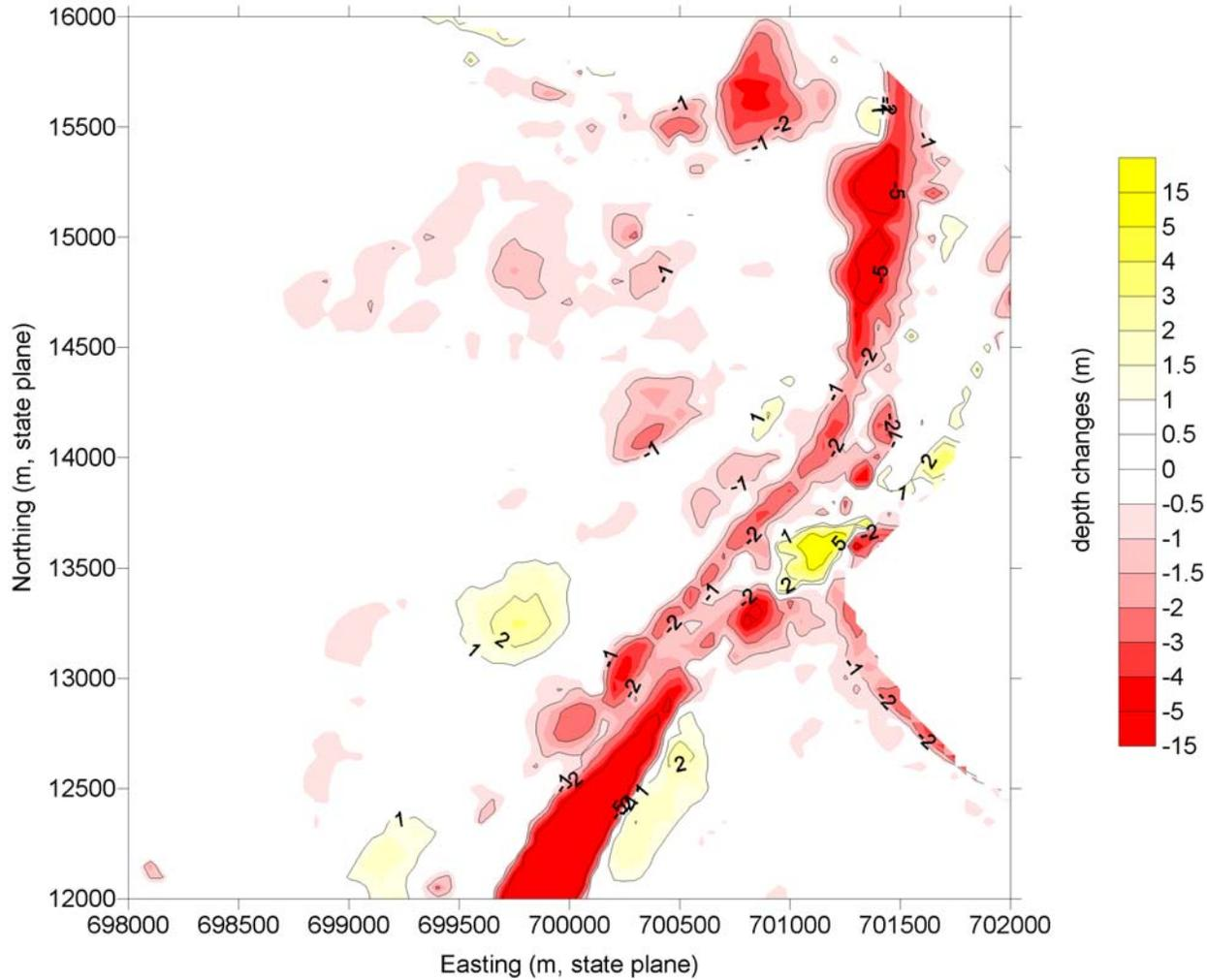
Figure 4.15 Change Map Showing a Deepening from 2000 to 2003 as negative and more shallow as positive in the tidal inlet region
