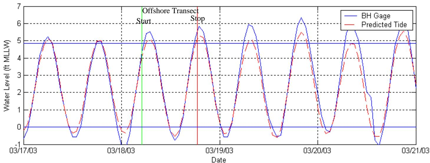
Figure 4.20 Predicted and observed water levels during the March 2003 ADCP survey (Offshore Transect)
