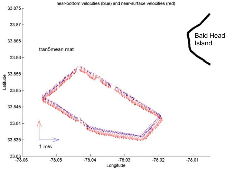
**Figure 3.49 Peak ebb current velocities at offshore transect for October 2000 ADCP survey**
