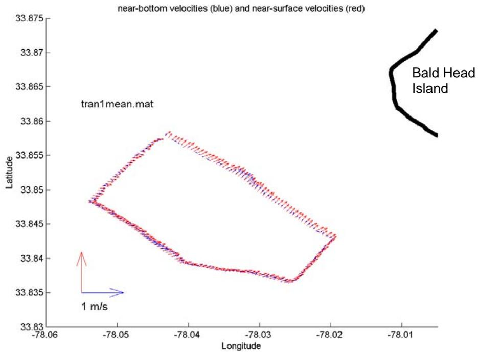
**Figure 3.50 Peak flood current velocities at offshore transect for October 2000 ADCP**
