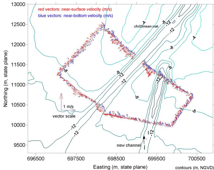
**Figure 4.29 Near-bottom flow field reversal on flood tide from April 2002 survey**
