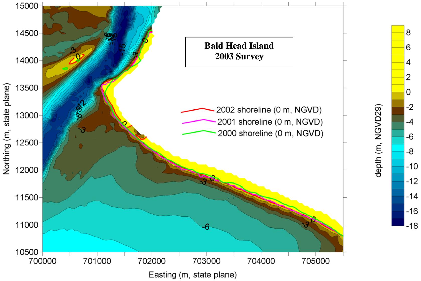
Figure 3.23 Inset of bathymetry along the western portion of Baldhead Island, 2003.
