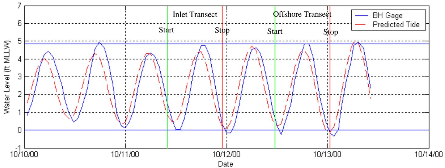
Figure 4.17 Predicted and observed water levels during the October 2000 ADCP survey
