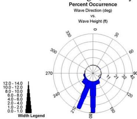
Figure 3.38 Wave Height Roses for FRF Gauges (2003).
