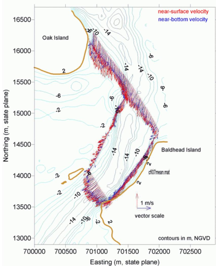
Figure 4.30 April 2002 ADCP survey at inlet transect during ebb flow.
