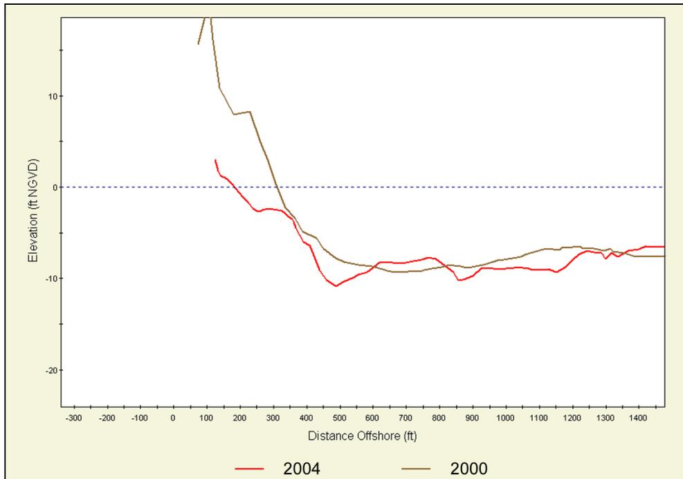
**Figure 3.7 On/Offshore Profile Bald Head Island STA 53+00**
