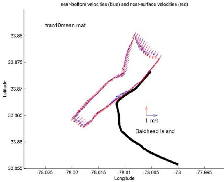
**Figure 3.47** Peak ebb current velocities at inlet transect for October 2000 ADCP survey
