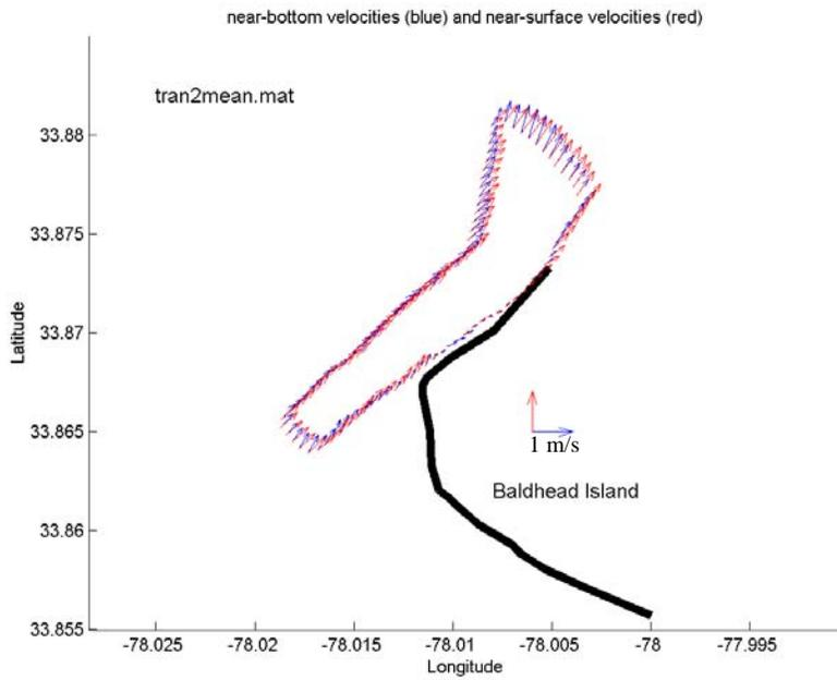
**Figure 3.48** Peak flood current velocities at inlet transect for October 2000 ADCP
