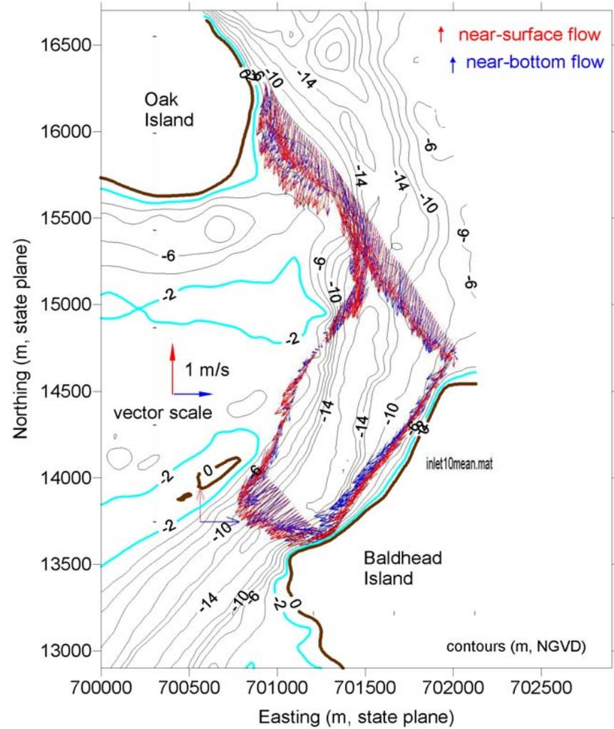
Figure 4.31 March 2003 ADCP survey at inlet transect during ebb flow.
