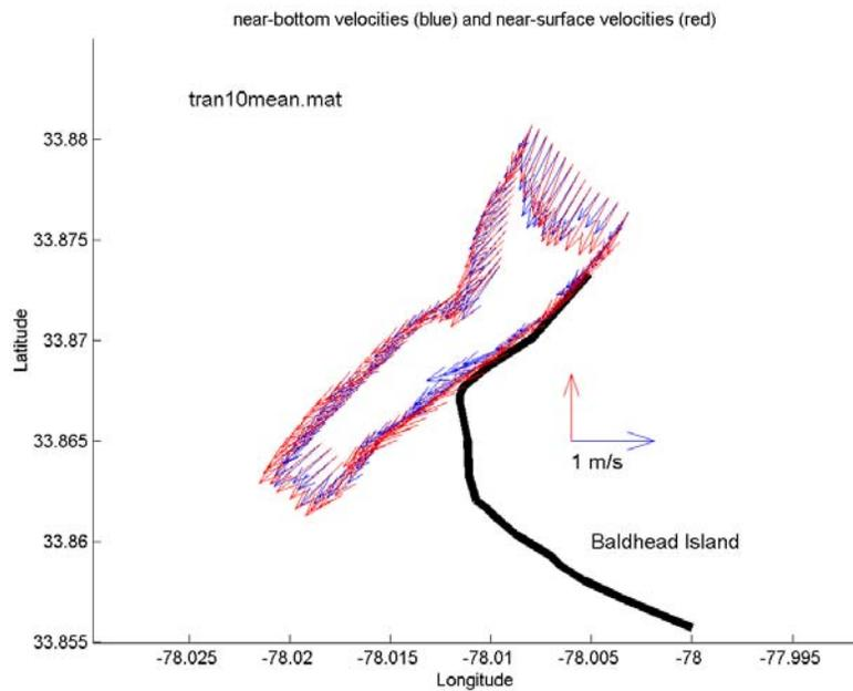
Figure 4.23 October 2000 ADCP survey at inlet transect during peak ebb flow. Note that survey transect does not cover same area as the April 2002 survey.
