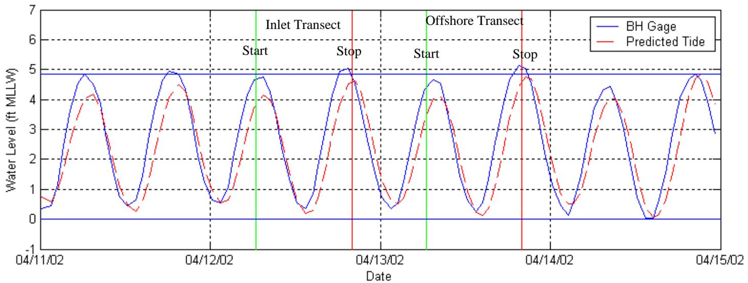
Figure 4.18 Predicted and observed water levels during the April 2002 ADCP survey
