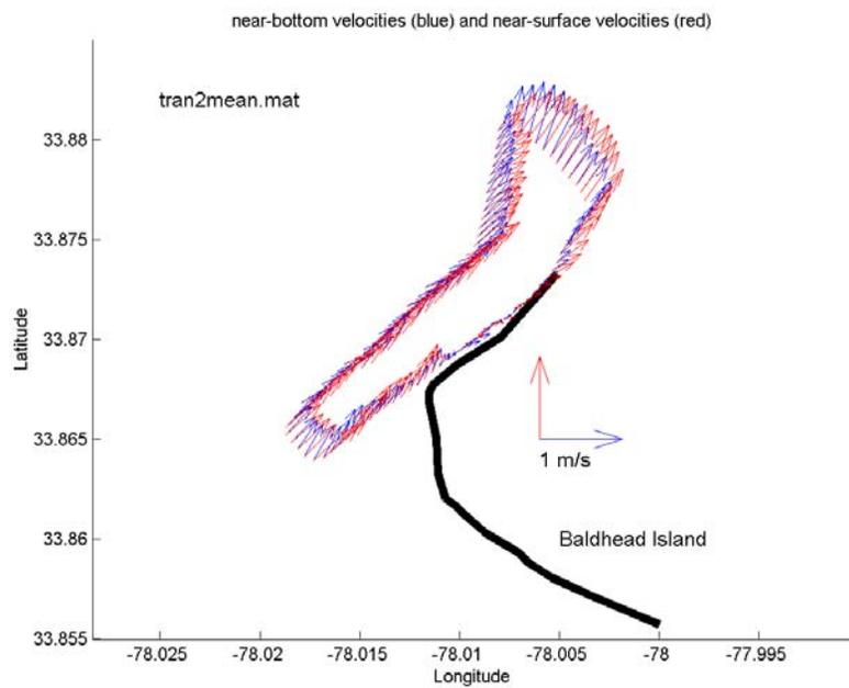
Figure 4.21 October 2000 ADCP survey at inlet transect during peak flood flow. Note that survey transect does not cover same area as the April 2002 survey.
