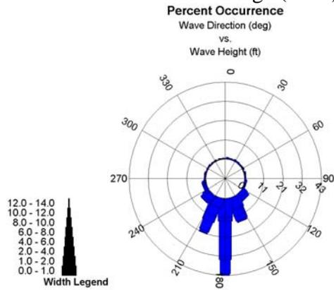
Figure 3.36 Wave Height Roses for FRF Gauges (2001).
