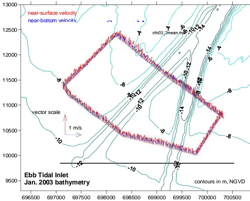
Figure 3.58 Peak flood current velocities at offshore transect for March 2003 ADCP survey
