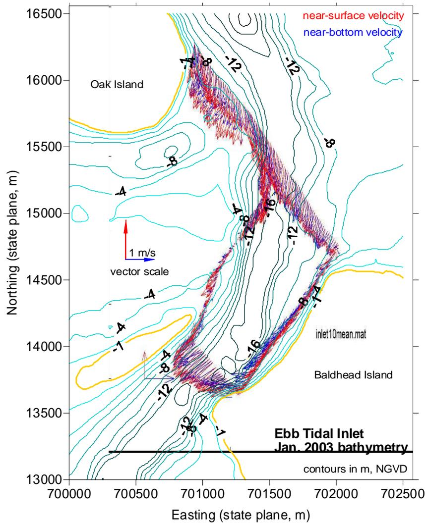
Figure 3.55 Peak ebb current velocities at inlet transect for March 2003 ADCP survey
