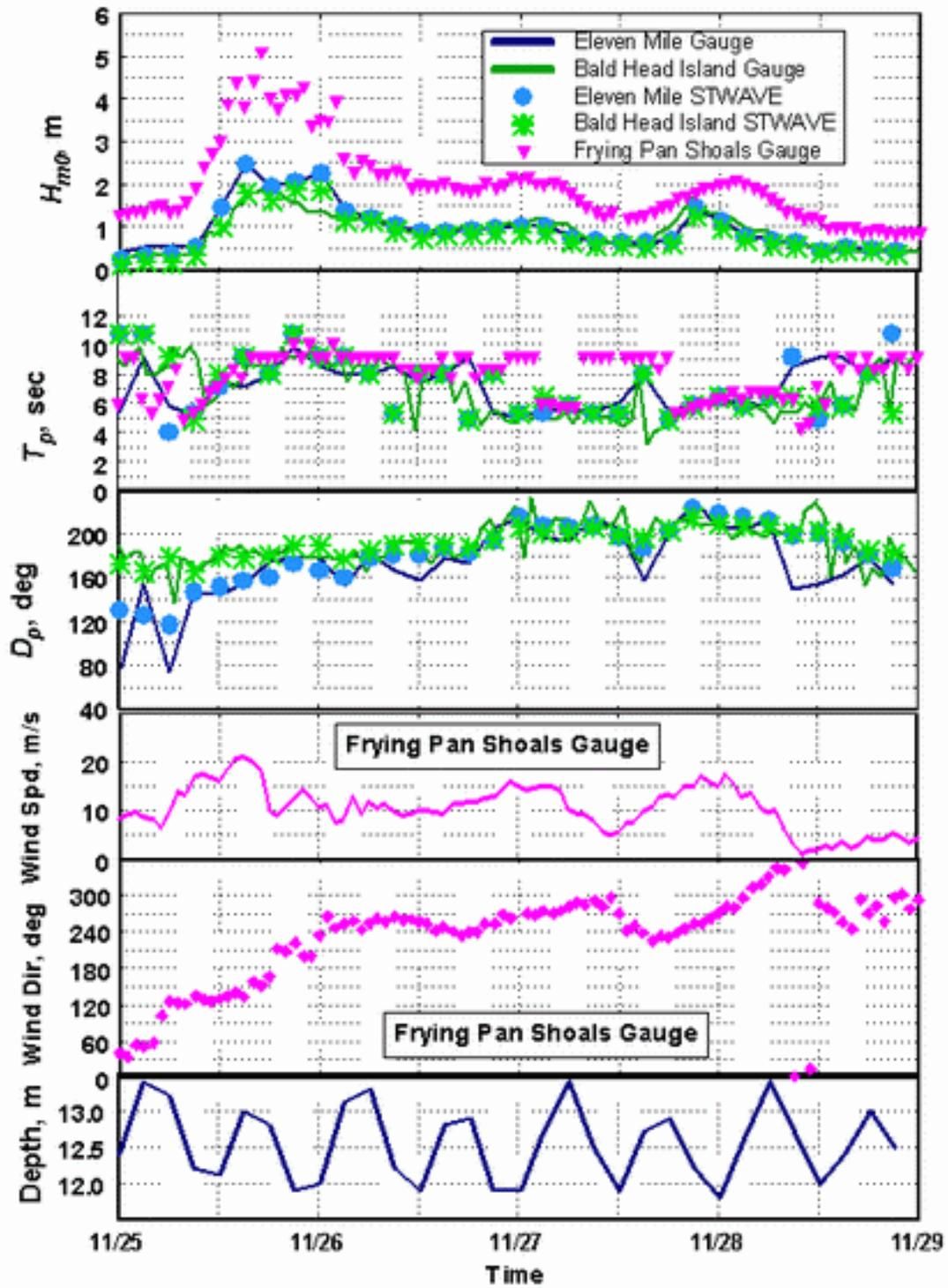
Figure 3.43 STWAVE Model Results Compared to Observed Gauge Data (Nov 2000 Storm).
