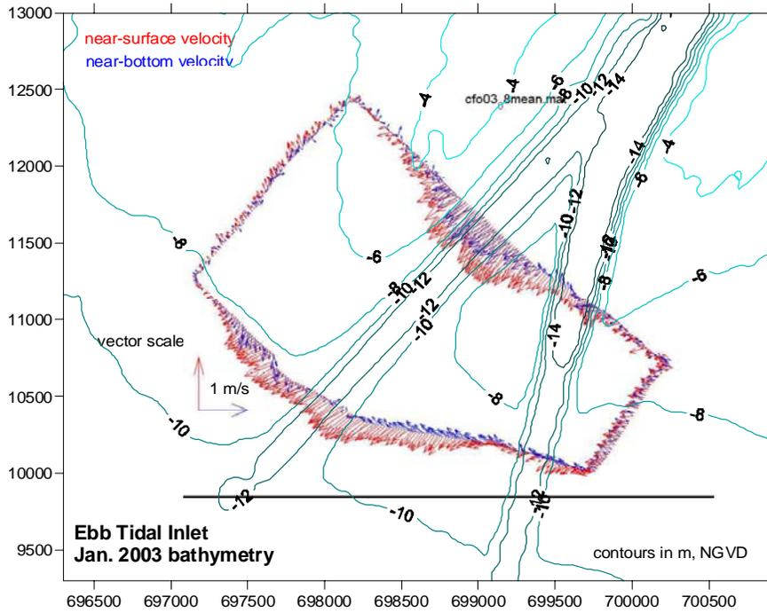
Figure 3.57 Peak ebb current velocities at offshore transect for March 2003 ADCP survey
