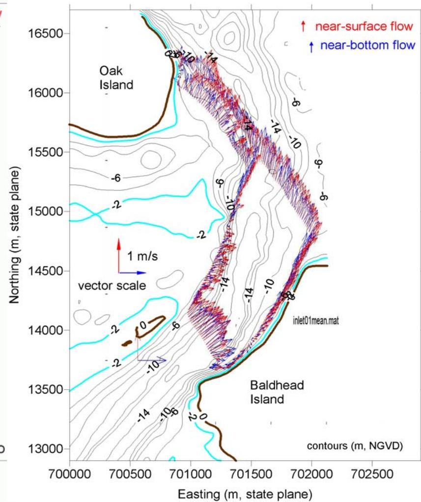
Figure 4.33 March 2003 ADCP survey at inlet transect during flood flow.
