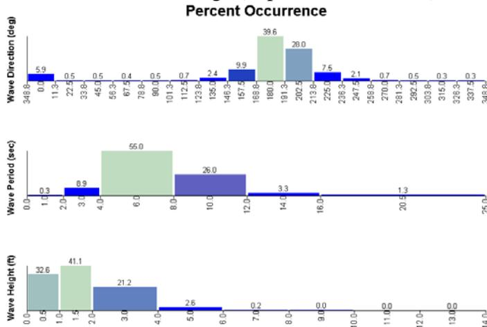
Figure 3.33 Wave Histograms for FRF Gauges throughout deployment.
