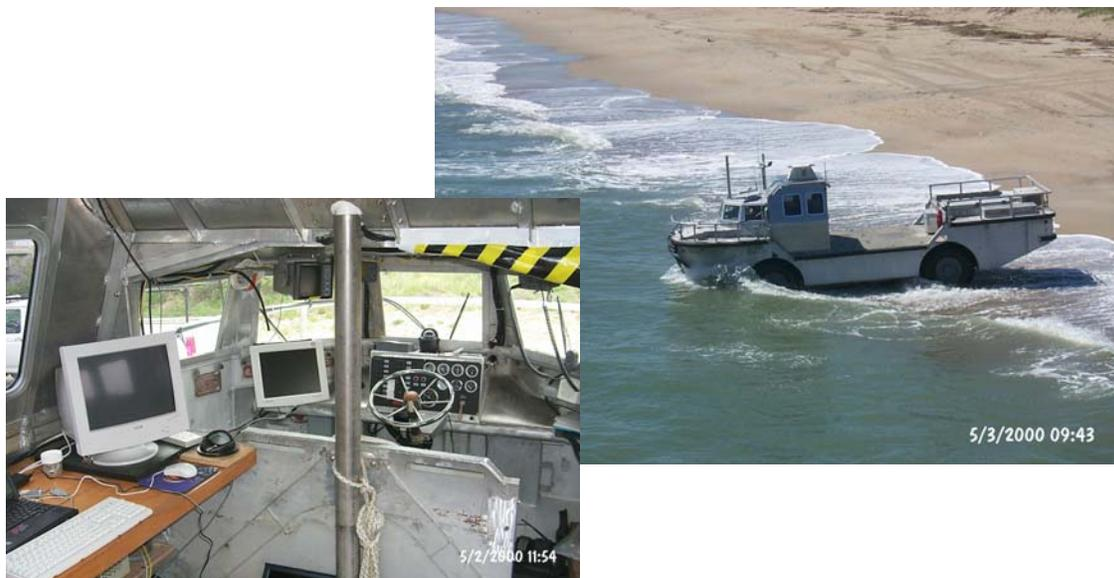
Figure 1.5 FRF Hydro-LARC Survey System
