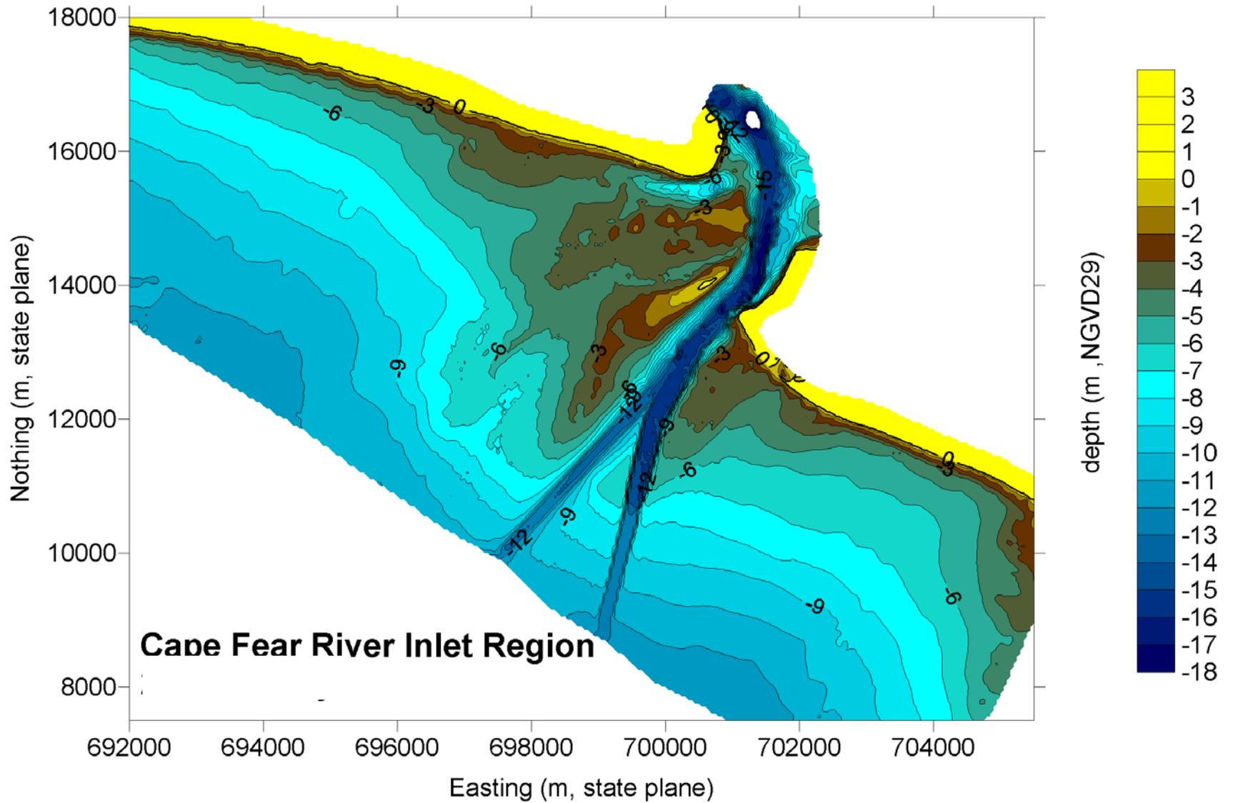
Figure 3.18 Bathymetry of the Cape Fear River Ebb Tidal Delta, 2003.
