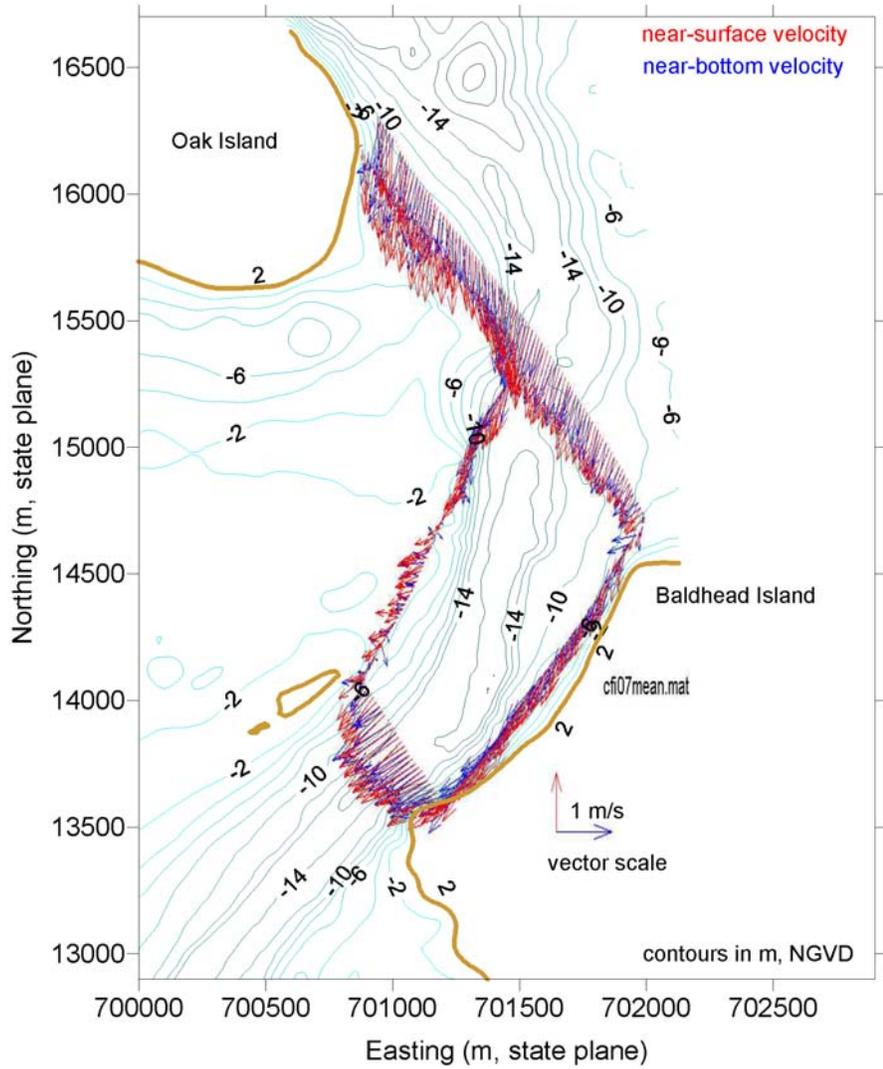
Figure 3.51 Peak ebb current velocities at inlet transect for April 2002 ADCP survey
