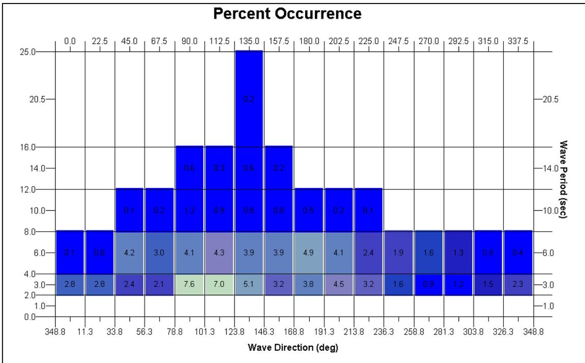
**Figure 3.31** Wave Period Block Diagram for WIS Level 3 Station 317.
