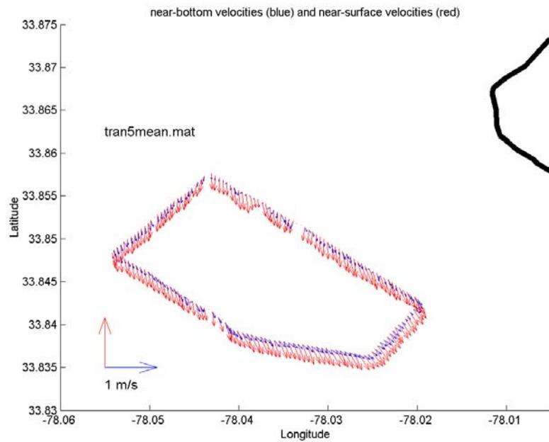
Figure 4.27 October 2000 ADCP survey at offshore transect during peak ebb flow.
