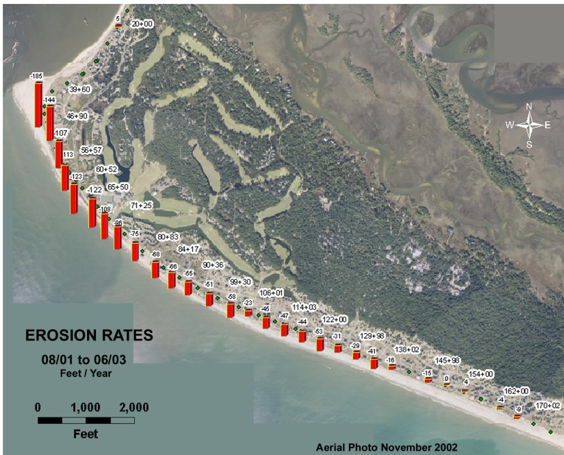
Figure 4.4 Bald Head Island Erosion Rates. August 01 to June 03
