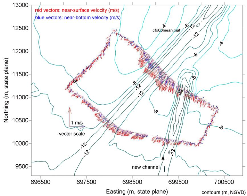
Figure 4.34 April 2002 ADCP survey at offshore transect during ebb flow.
