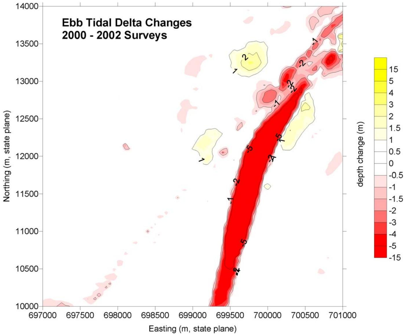
Figure 4.16 Change Map Showing a Deepening from 2000 to 2003 as negative and more Shallow as positive in the new channel region.
