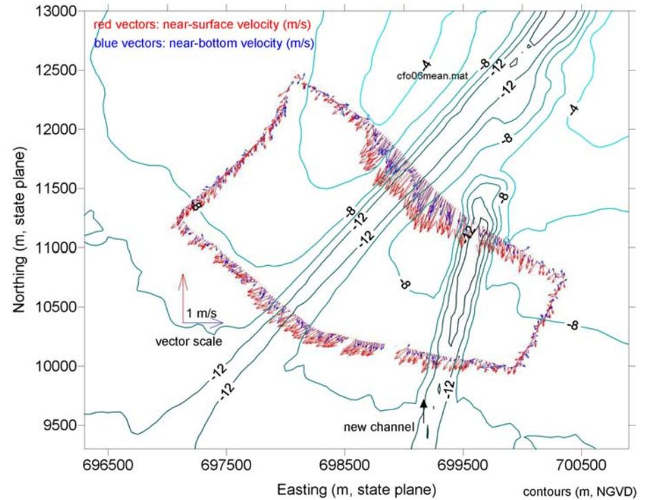
Figure 4.28 April 2002 ADCP survey at offshore transect during peak ebb flow.
