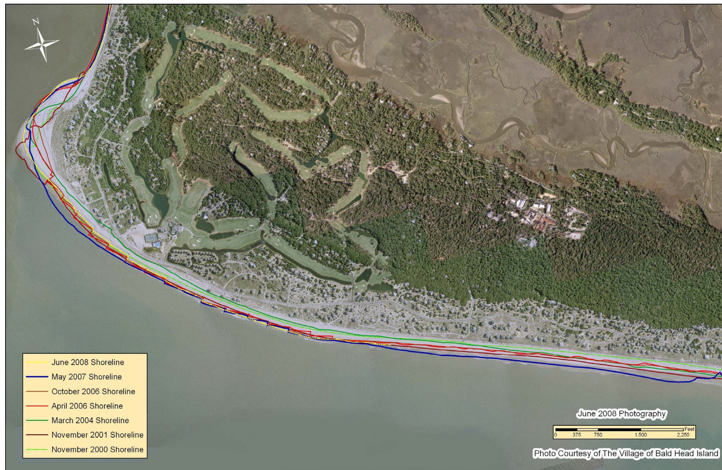
Figure 4.12 Shoreline Comparison: Pre and Post groin field reconstruction and beach disposal
