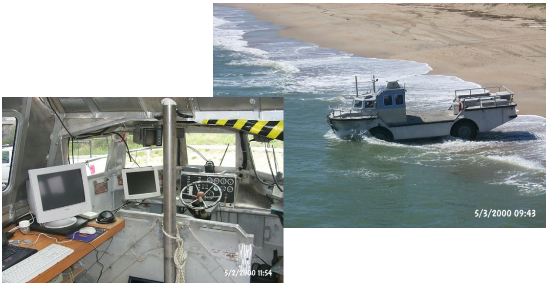
Figure 1.5 FRF Hydro-LARC Survey System
