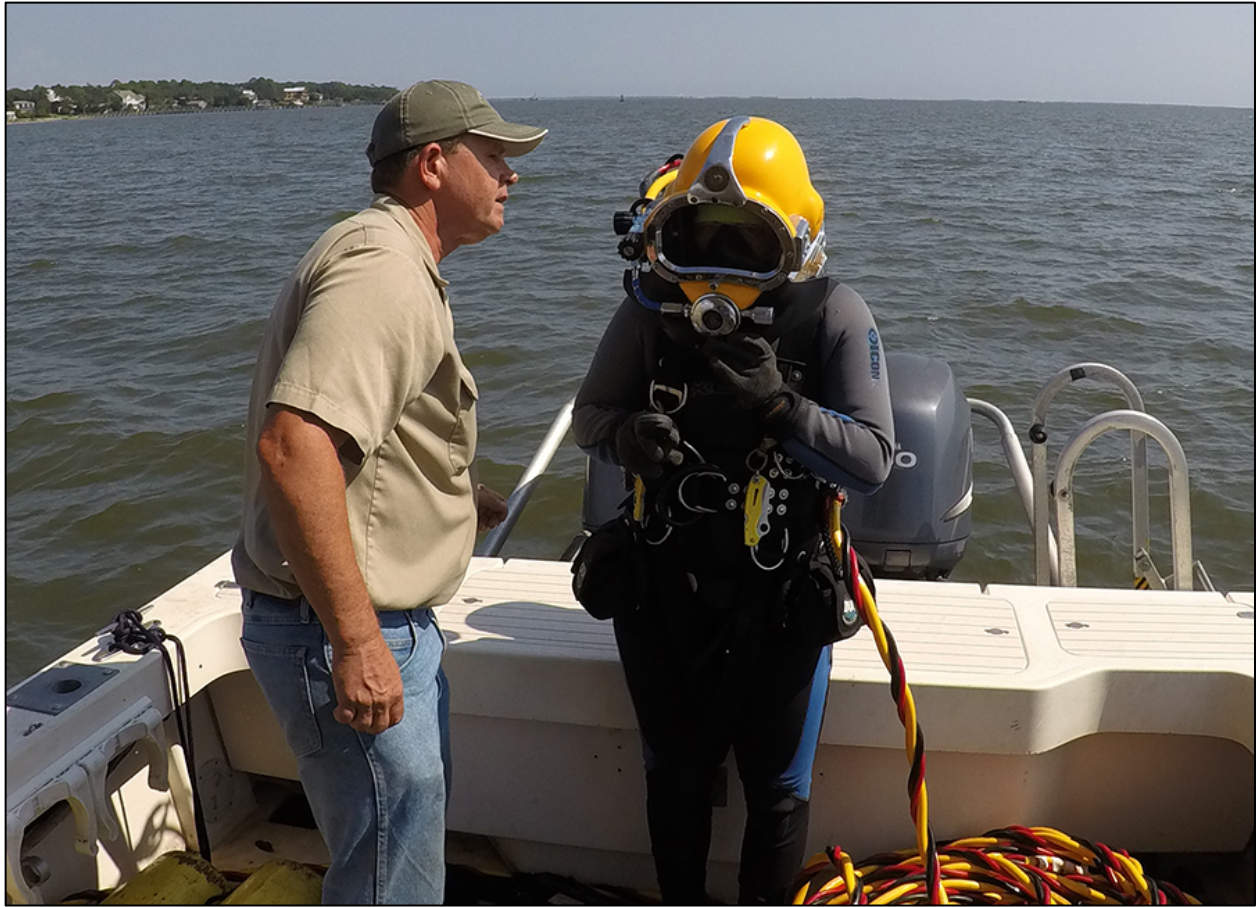
Figure 3-26. Surface Supplied Air-equipped diver Ms. Loren Clark and tender James Duff; note the black pneumo hose on the diver's umbilical, which is employed for depth readings in low and zero visibility environments; yellow hose is air; red is communication line.
