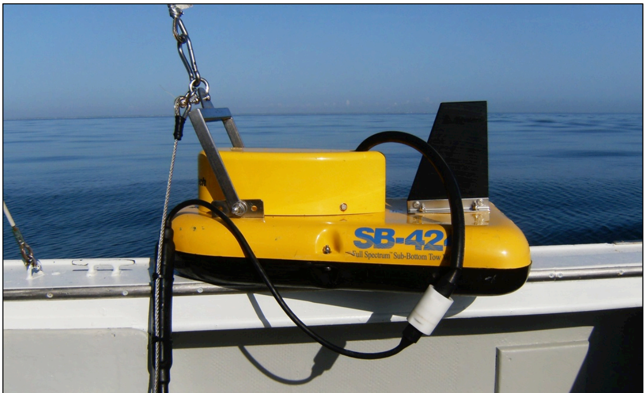
Figure 3-08. The EdgeTech SB-424 towfish employed during the survey.
