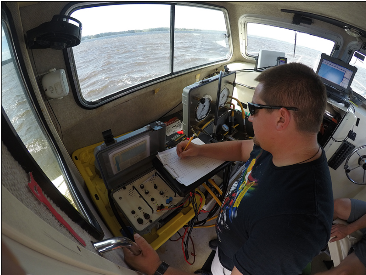
Figure 3-27. Dive Supervisor Mr. Jeff Pardee manning the dive station that includes diver communications and air manifold with pneuemo gauges for depth readings.
