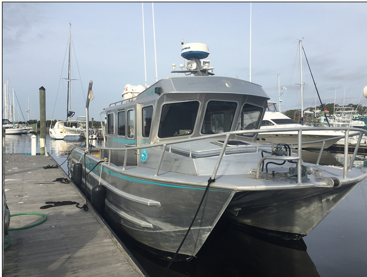
Figure 3-11. The R/V Seahawk , a 34-foot aluminum-hulled catamaran employed for the survey of the Offshore Area.
