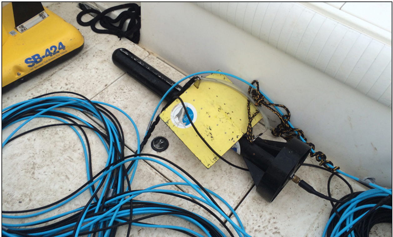
Figure 3-07. Marine Sonic Technology HDS sidescan sonar with 800/900-kilohertz towfish employed during the survey.
