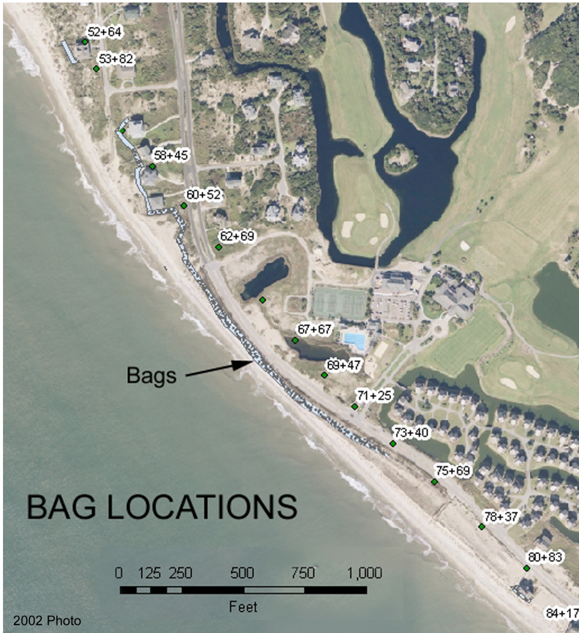
Figure 4.7 Sand Bag Locations along Bald Head Island South Beach.
