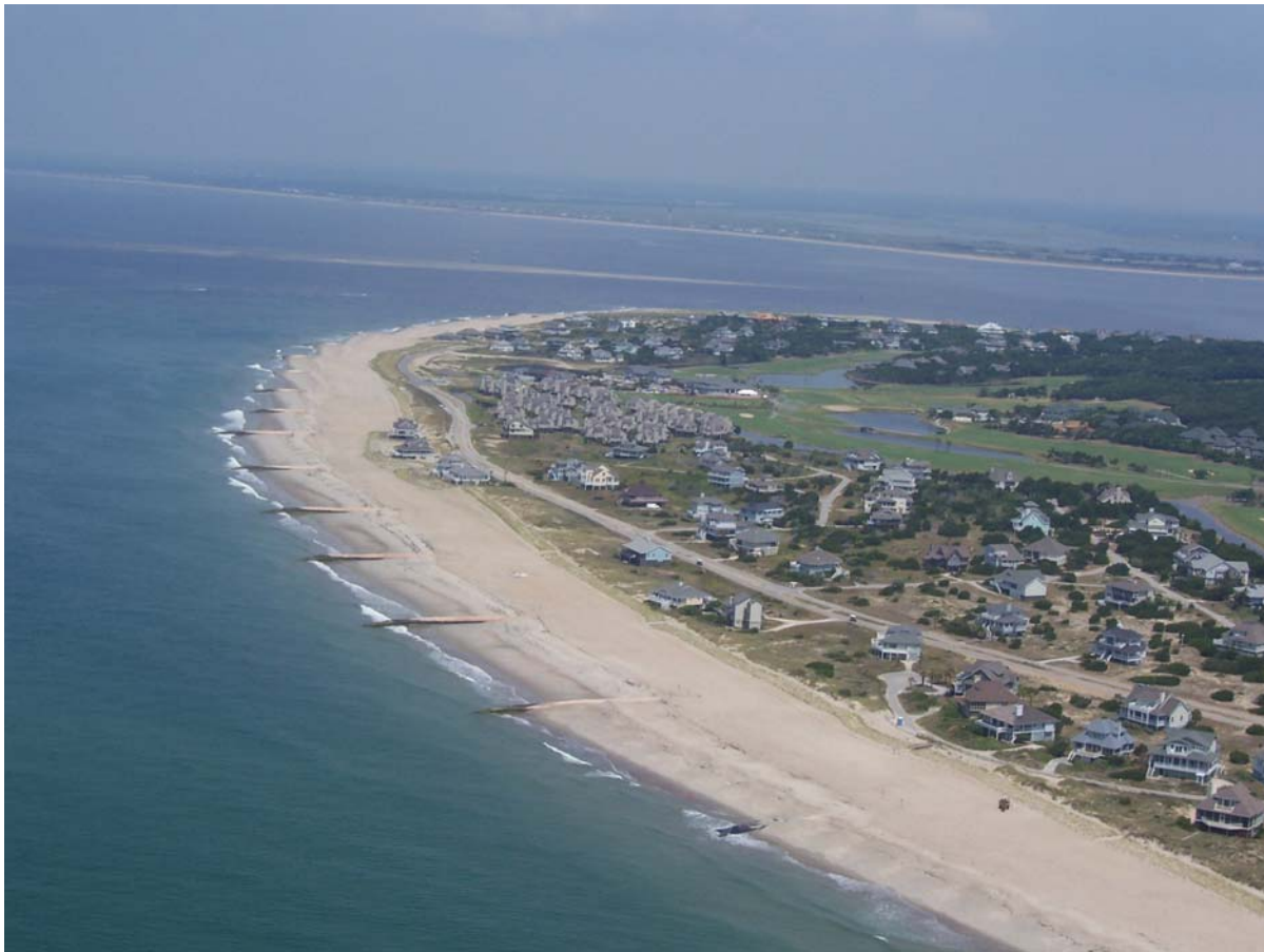
Figure 2.4 Reconstructed Groinfield along Bald Head Island, July 2006 (Courtesy of Village of Bald Head Island)
